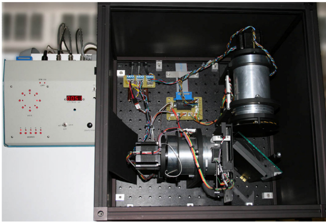
Figure 2 The chFP device designed and built for use during this study used to measure MPOD along 4 radii at 0°, 2°, 4° and 6° eccentricities.
